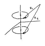
The quantities  $\int_{\phi'=0}^{2\pi} \left(\frac{1}{R_1} - \frac{1}{R_2}\right) \operatorname{Iasin} \phi' d\phi' \text{ and } \int_{\phi'=0}^{2\pi} \left(\frac{1}{R_1} - \frac{1}{R_2}\right) \operatorname{Iacos} \phi' d\phi'$
