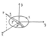
$$A = \int_{\phi=0}^{2\pi} \frac{\mu_0 I_0 a d\phi' \cos \omega \left(t - \frac{|x-x'|}{v}\right)}{4\pi |x-x'|} \left(-\sin \phi' \frac{i}{2}x + \cos \phi' \frac{i}{2}y\right)$$
