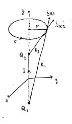
4.23. To enaluate  $\nabla \times B$  at a point on the xy plane, we have to first find  $\nabla \times B$ at an arbitrary point  $(r, \phi, 3)$  and then let  $3 \rightarrow 0$ . Generalizing the result of Problem 4.18, we have B(r, 0, 3) = 40 900 [r2+(vot-3)2]3/2 ~ 0
