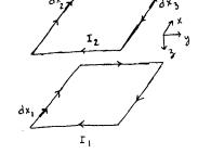
$$\frac{F_1}{4} = -\frac{M_0 I_1 I_2}{4\pi} \int_{X_2 = 0}^{\alpha} \int_{X_1 = 0}^{\alpha} \frac{dx_1 dx_2 [(x_1 - x_2) \dot{x}_x + d \dot{x}_3]}{[(x_1 - x_2)^2 + d^2]^{3/2}}$$
