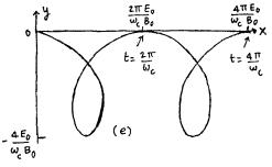
4.5. Writing the equations of motion of the test charge and eliminating  $v_y$ , we get  $\frac{d^2V_x}{dt^2} + w_c^2v_x = \frac{9E_0}{m}w_c \cos wt$
