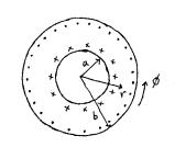
But from  $V(3,t) = \int_{r=a}^{b} E_{r}(r,3,t)$  and since  $E_{r} \propto \frac{1}{r}$  from Gauss' law, we have  $E_{r}(r,3,t) = \frac{V(3,t)}{r \ln \frac{b}{a}}$ . Also, from  $I(3,t) = \int_{g=0}^{2\pi} H_{g}(r,3,t) r d\phi$ ,
